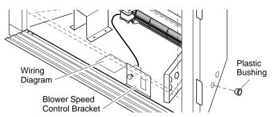
Figure 33 - Installing Plastic Bushing and Wiring Diagram Sticker
